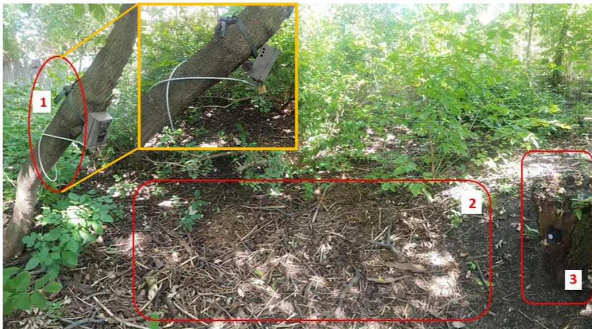
Figure 2. An example site setup. (1) Wrap cords to keep them tight against the tree. Use pieces of wood to prop the camera at the correct angle; (2) Choose a site that has minimal vegetation between the camera and the [optional] lure to prevent windblown vegetation from falsely triggering the camera; (3) Ensure a stable object (tree, pole, fence, etc.) is within 3-5 meters of the camera to use for holding the [optional] lure in place.
