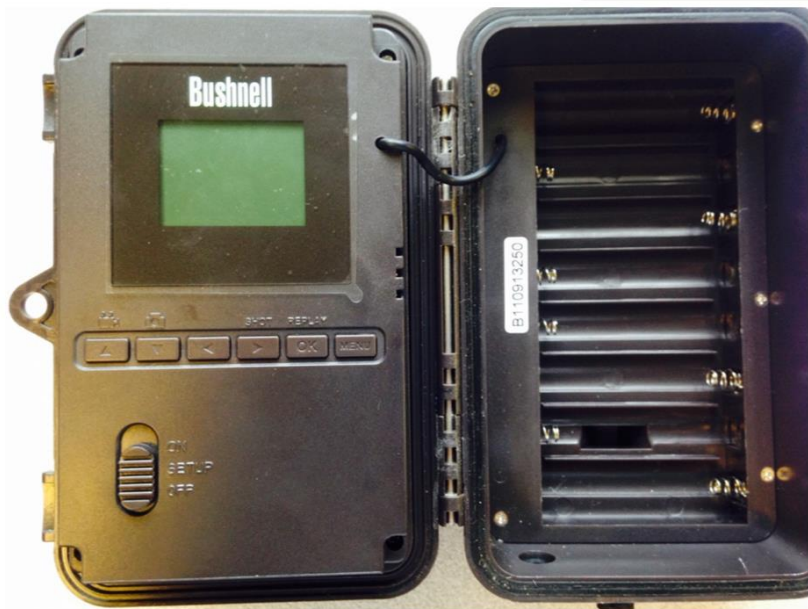
Figure 8. Interior of Bushnell TrophyCam
